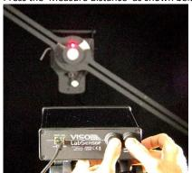
The glass surface of the lamp produces a lot of internal reflections of the laser beam, and it complicates the exact distance calculation. The precise distance determination is essential in achieving the best results. That is why a fixed white target point was designed above the lamp luminous area.
